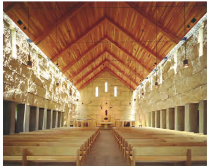
The monastic church rises 40 feet high and covers an area of about 5,800 square feet. It is constructed of 427 huge blocks of Texas limestone, each weighing 4000–5000 pounds, that are held in place by thick mortar and the compression of their own weight.
